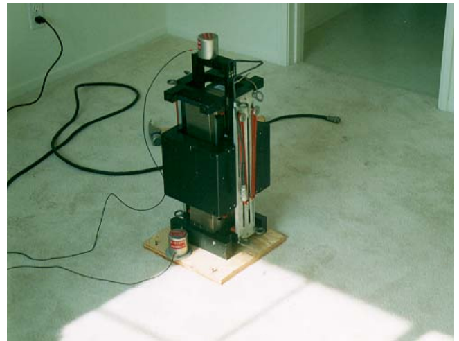
Figure 1 - Frequency Controlled Oscillating Mass Used to Measure Frequency Response in Floors
